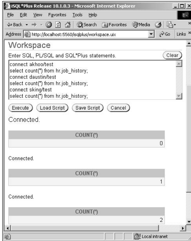
Figure 5-5: Different users may see different data from a view with a dynamic WHERE clause.
